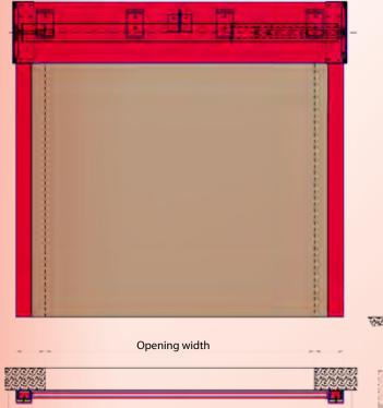
Special construction: space requirement for installation = opening width + 23.6"
