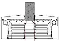
Installation of the housing directly to the wall
