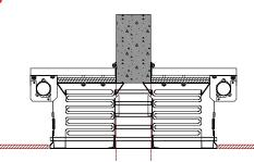
Installation of the housing directly to the wall, false ceiling is attached to the housing on both sides
